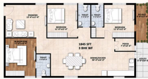
FLAT 2 & 3 CARPET AREA 1288.32 SFT BALCONY AREA 88.05 SFT COMMON AREA 468.63 SFT SUPER BUILT AREA 1845 SFT
