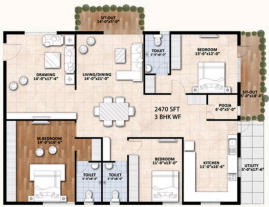
FLAT 1 CARPET AREA 1703.49 SFT BALCONY AREA 163.71 SFT COMMON AREA 602.8 SFT SUPER BUILT AREA 2470 SFT
