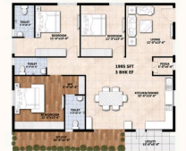
FLAT 11 & 12 CARPET AREA 1353.45 SFT BALCONY AREA 143.80 SFT COMMON AREA 497.75 SFT SUPER BUILT AREA 1995 SFT
