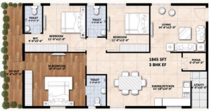
FLAT 16 CARPET AREA 1240.22 SFT BALCONY AREA 137.67 SFT COMMON AREA 467.11 SFT SUPER BUILT AREA 1845 SFT
