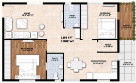
FLAT 13 & 14 CARPET AREA 896.52 SFT BALCONY AREA 59.09 SFT COMMON AREA 339.39 SFT SUPER BUILT AREA 1295 SFT
