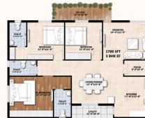
FLAT 10 CARPET AREA 1187.47 SFT BALCONY AREA 76.10 SFT COMMON AREA 436.43 SFT SUPER BUILT AREA 1700 SFT
