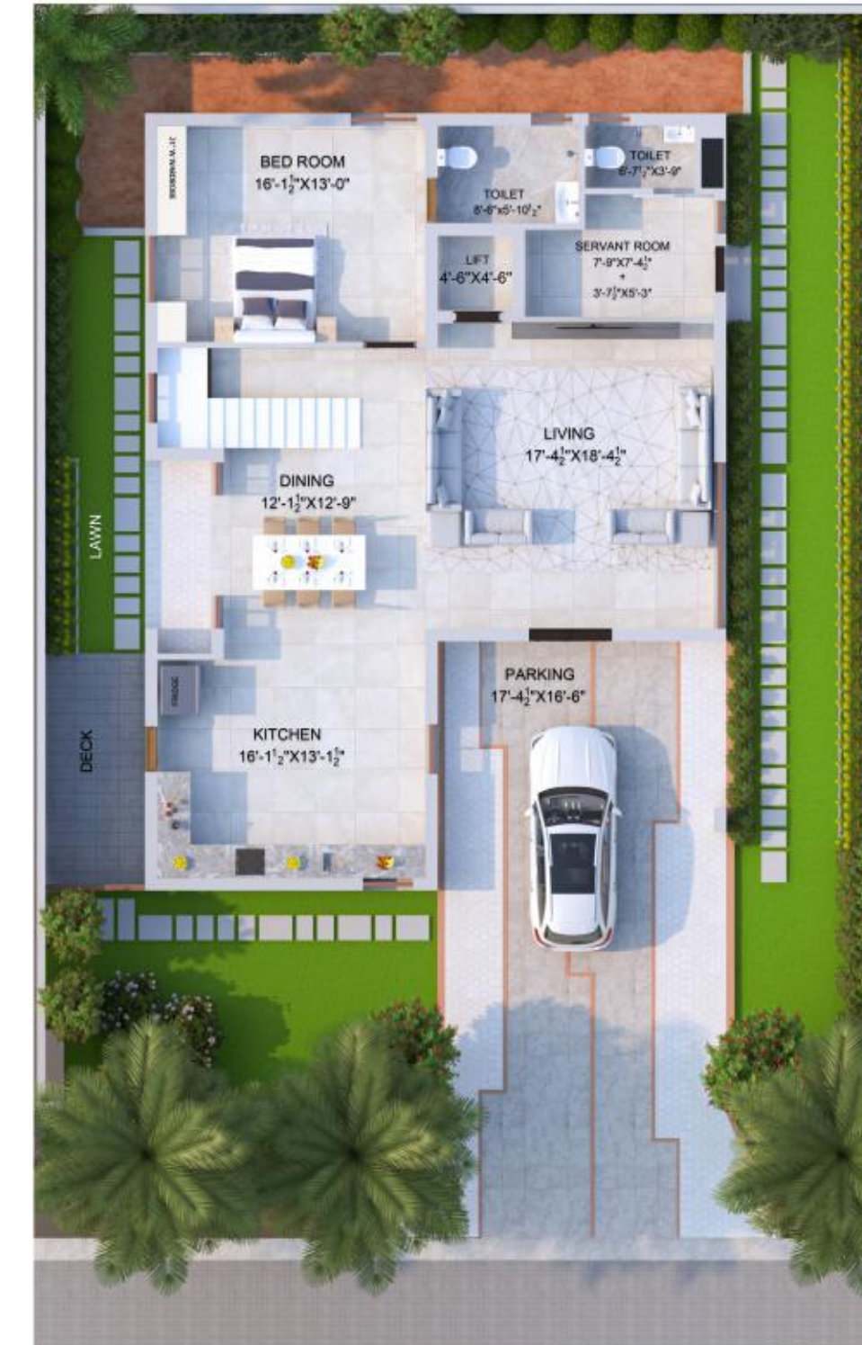
GROUND FLOOR PLAN
